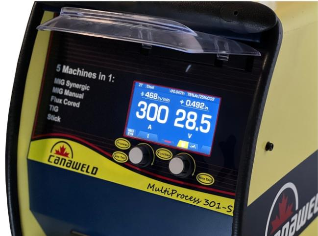
A synergic welding machine helps workers to work quickly without making mistakes and always with high-quality standards. The most advanced digital generators for welding can have selectable memories where all the settings are ready to go, depending on the material to be welded, the diameter of the wire used, and the gas chosen to shield the weld pool from oxidation.
